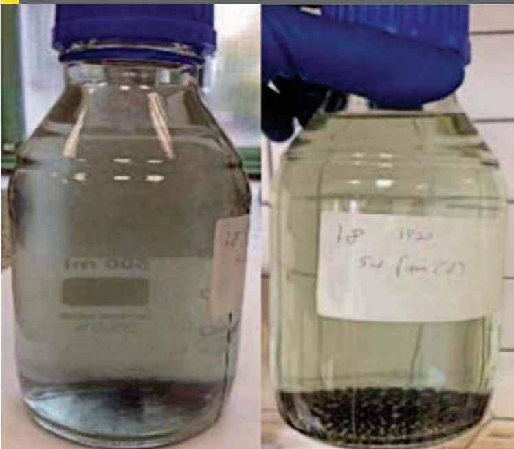
Fig 12: Solids precipitating out of sour water after 12 hours
