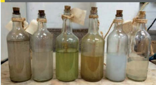
Fig 3: Water quality in feed and effluent of an FCC (L), Coker (C) & HT (R) SWS
