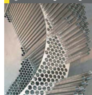
Fig 8: NORAM RF™ gas exchanger
