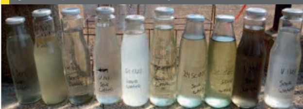
Fig 3: Water quality in feed and effluent of an FCC (L), Coker (C) & HT (R) SWS
