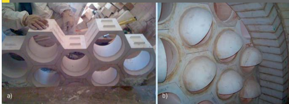
Fig 5: MECS® VectorWall™ ceramic furnace internals
