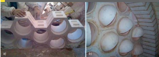
Fig 5: MECS® VectorWall™ ceramic furnace internals
