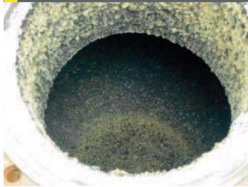
Fig 4: Compact material found on the top of the catalyst of the first converter
