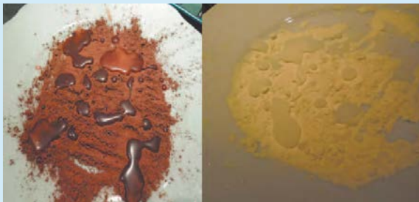
Fig. 8: Water "beads" when sprayed on cocoa (left) and sulphur dust (right).
