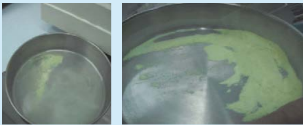
Figs. 5 & 6: Granular sulphur particulate: Sub-50 mesh, 300 micron (0.3mm), Odessa.
