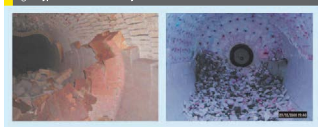
Fig 1: Typical extreme refractory failures
