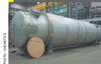
Fig 5: Chemetics radial flow cold heat exchanger ready for shipment
