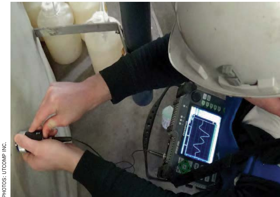
UTComp monitoring of a FRP tank.
