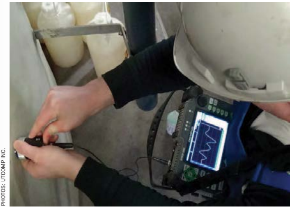
UTComp monitoring of a FRP tank.
