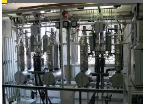
Fig 6: Reactors used for catalyst stage tests
