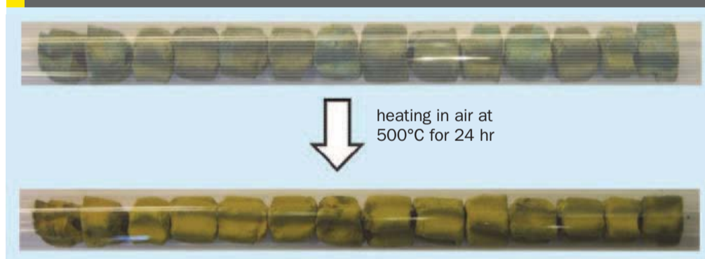
Fig 11: Colours alone cannot be used for assessment of the catalyst performance. Here reduced vanadium is reoxidised by heating of a greenish sample in air
