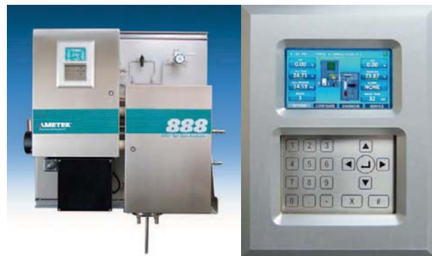
The Model 888 sulphur analyser.
