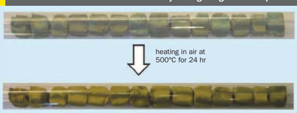
Fig 11: Colours alone cannot be used for assessment of the catalyst performance. Here reduced vanadium is reoxidised by heating of a greenish sample in air
