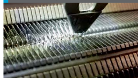
Fig. 13: Detail of knitting process in catalyst gauze manufacturing
