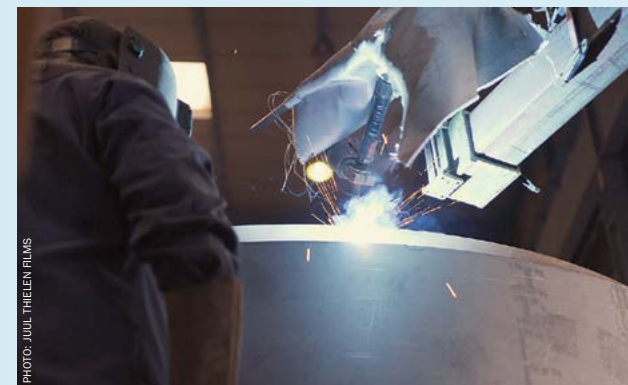
Welding of the HP stripper at SBN's manufacturing site in Ternitz, Austria.
