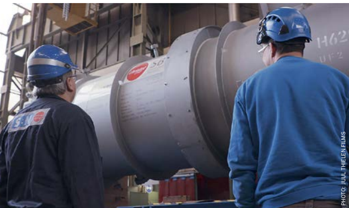
New Safurex® HP stripper ready for shipment at SBN, Austria.
