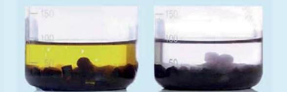
Fig. 18: Chromium VI visible in ShiftMax 120 (L); absent in ShiftMax 120 HCF (R)
