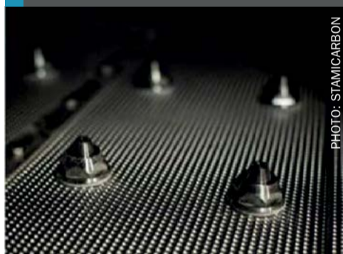
Fig. 1: Stamicarbon's film spraying nozzles
