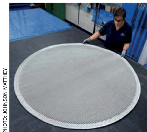
Fig. 1: HICON – PGM gauze pack for HP nitric acid plant.
