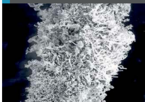
Fig. 11: SEM of Ca-contaminated Pt-Rh wire (magnification x200)
