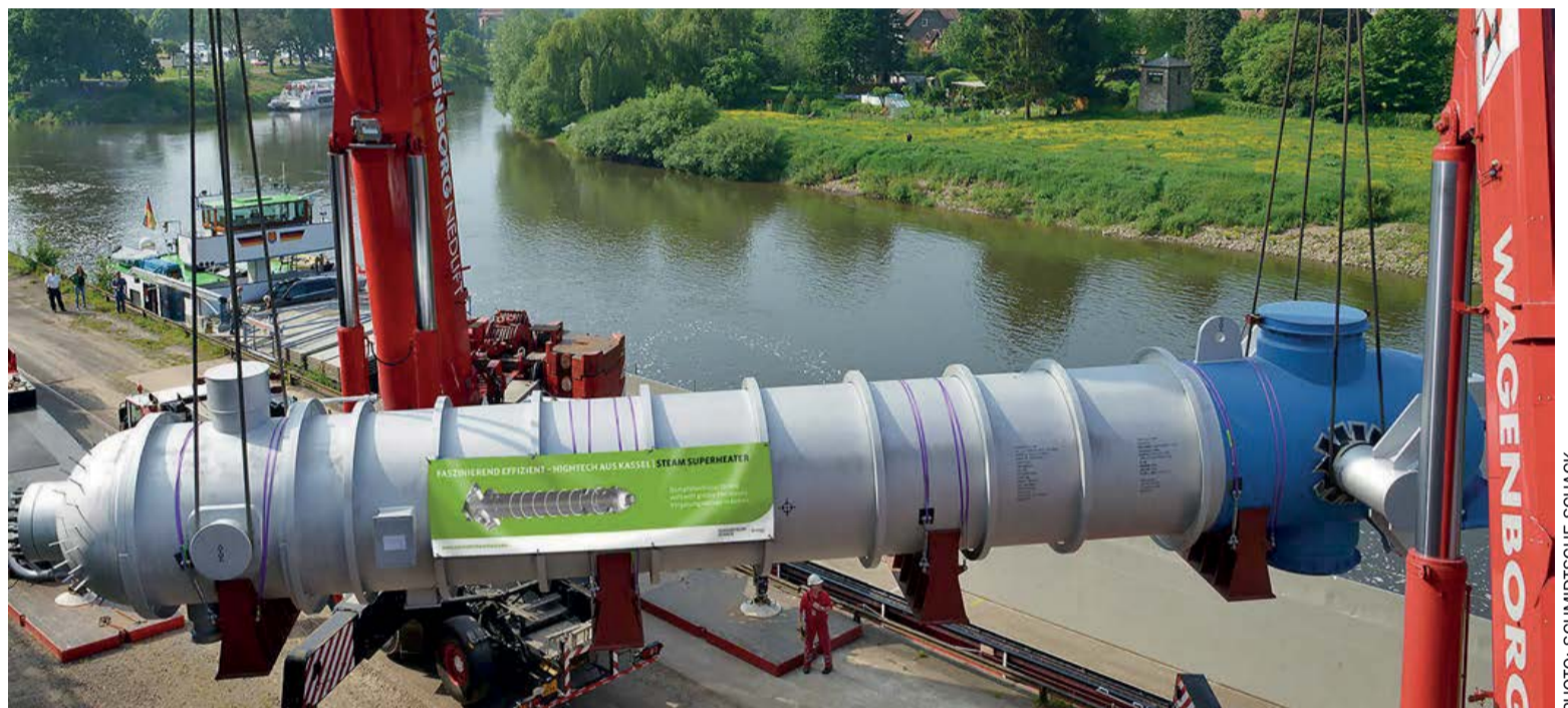
High performance steam superheater ready for shipment.
