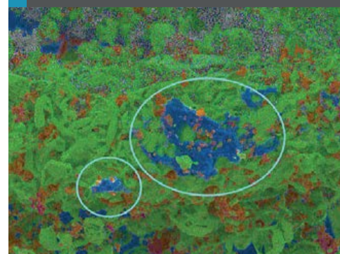
Fig. 10: EDX spectroscopy/mapping of a surface deactivated by carbon
