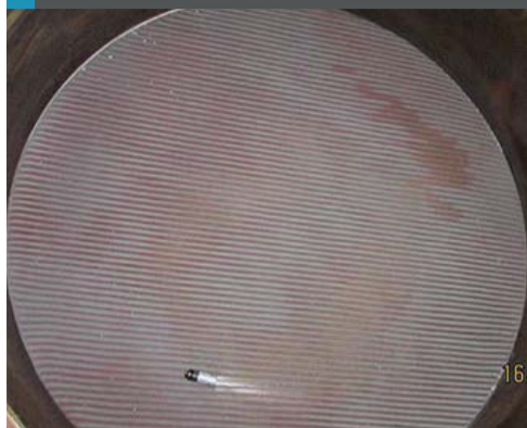
Fig. 8: Deactivated catalyst surface by iron contamination
