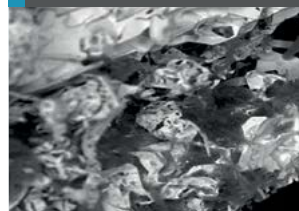
Fig. 12: SEM of Mg-contaminated Pt-Rh wire (magnification x200)
