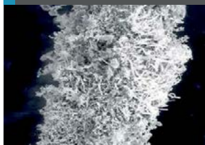
Fig. 11: SEM of Ca-contaminated Pt-Rh wire (magnification x200)
