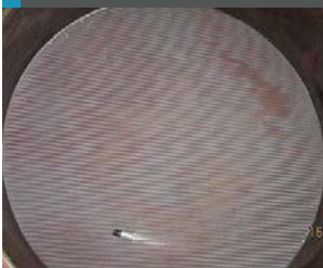
Fig. 8: Deactivated catalyst surface by iron contamination
