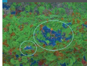
Fig. 12: SEM of Mg-contaminated Pt-Rh wire (magnification x200)
