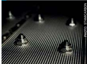
Fig. 1: Stamicarbon's film spraying nozzles
