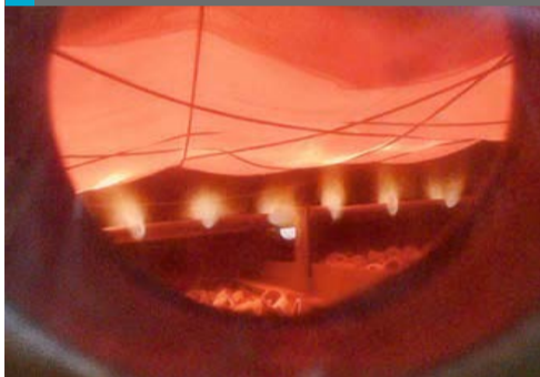
Fig. 22: Homogeneous ignition over the entire catalyst surface
