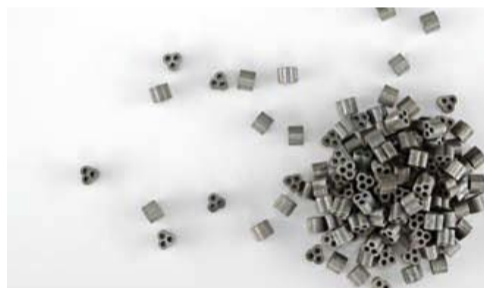
Above left: EnviCat N 2 O catalyst, iron on zeolites; Above right: EnviCat N 2 O catalyst, cobalt/manganese on alumina.
