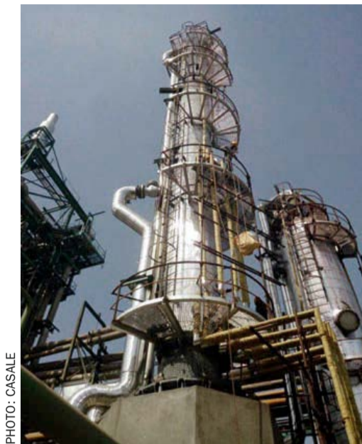
Fig. 1: New process condensate stripper
