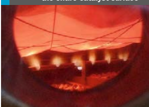
Fig. 22: Homogeneous ignition over the entire catalyst surface
