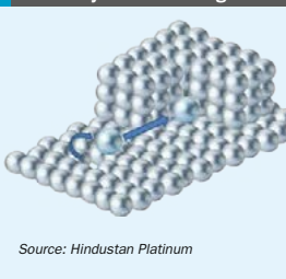
Fig. 14: Restructuring of the surface by thermal etching schematic
