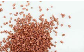
Above left: EnviCat N 2 O catalyst, iron on zeolites; Above right: EnviCat N 2 O catalyst, cobalt/manganese on alumina.
