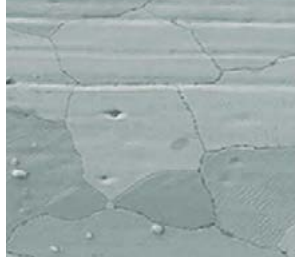
Fig. 11: STM image of Pt/Rh surface after annealing to a temperature of 700°C (Pt/Rh = dark/bright dots)
