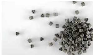
Above left: EnviCat N 2 O catalyst, iron on zeolites; Above right: EnviCat N 2 O catalyst, cobalt/manganese on alumina.
