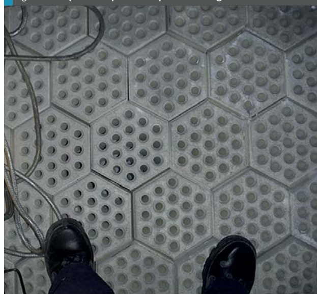
Fig. 15: Post operation inspection of Topsoe HTZR™ target tiles
