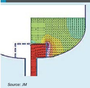
Fig. 10: STREAMLINE flow modelling of shift reactor
