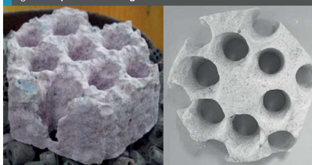
Fig. 9: Condition of KATALCO 94-1ZT target tile after service
