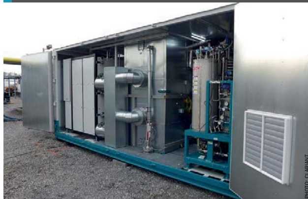
Fig. 3: LOHC installation – easy and safe hydrogen storage
