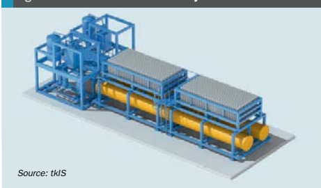
Fig. 7a: 3D model of 5 MW electrolysis skid
