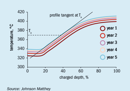
Fig. 13: HTS optimisation via remote monitoring
