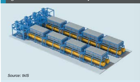
Fig. 7b: 3D model of 20 MW electrolysis skid
