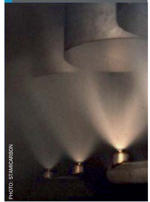
Fig. 6: MicroMist™ Venturi scrubbing
