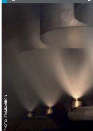
Fig. 6: MicroMist™ Venturi scrubbing
