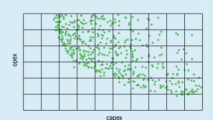
Fig. 5: Rapid evaluation of single-stage WCR concepts to select optimal opex and capex for a small-scale MeOH unit (depending on market conditions and customer requirements)
