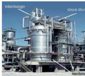
Fig. 8: Air Liquide's Lurgi WCR
