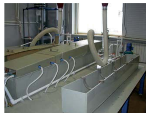
Fig. 4: The new section for the gauzes electrochemical activation
