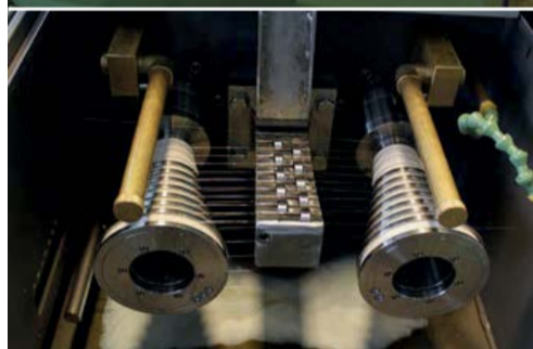
Fig. 2: Equipment for wire drawing and annealing
