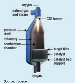
Fig. 6: Topsoe ATR reformer
