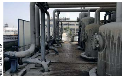
Fig. 4: Heat exchangers (left) and buffer vessels for the pumps (right) which are filled with weak acid from the absorption process from nitric acid Line II.
