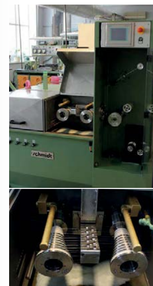
Fig. 2: Equipment for wire drawing and annealing
