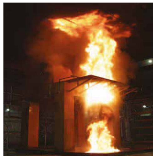
Fig. 2: Three-dimensional oil spill fire test.
