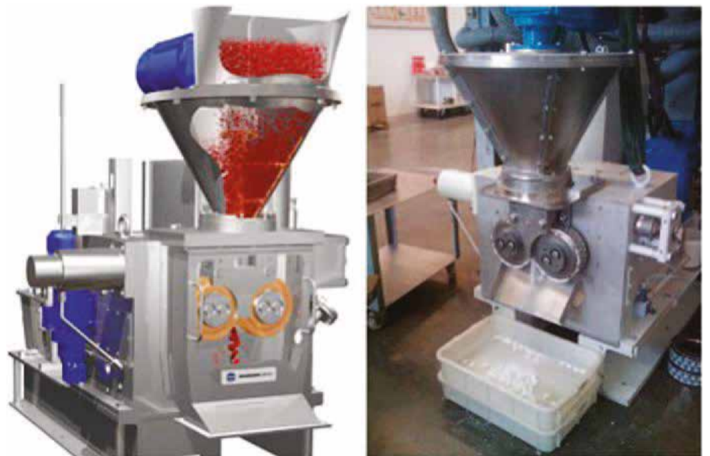
Fig. 10: Compacting equipment for production of super granules.
