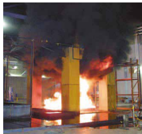
Fig. 3: Oil pool fire test.
