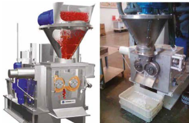
Fig. 10: Compacting equipment for production of super granules.
