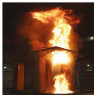
Fig. 2: Three-dimensional oil spill fire test.
