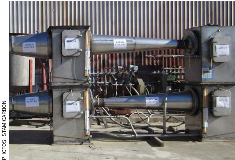
Fig. 12: Pilot Jet Scrubber during fabrication at ECI shop.
