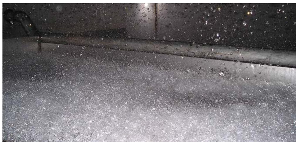
Fig. 4: Wetted DOI tray, showing intimate gas-water contact.
