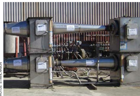
Fig. 12: Pilot Jet Scrubber during fabrication at ECI shop.
