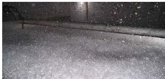
Fig. 4: Wetted DOI tray, showing intimate gas-water contact.
