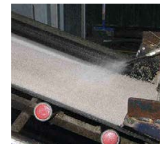
Fig 16: Stamicarbon Advance™ Coating Technology is applied to stabilise the prills before storage.
