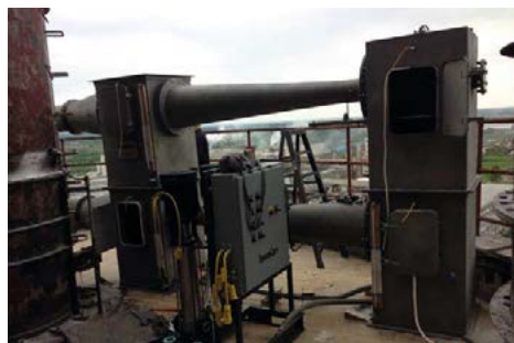
Fig. 13: Pilot Jet Scrubber located on top of prilling tower for emissions testing.
