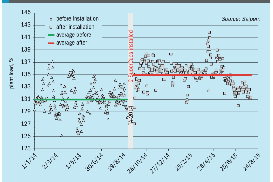
Fig 5: FFC: plant load before and after SuperCups installation
