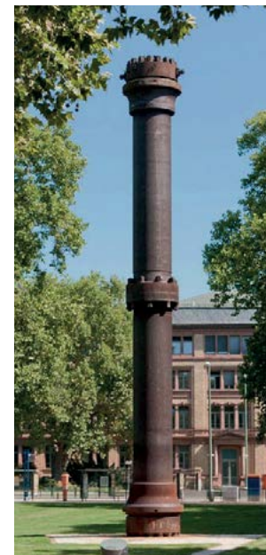
The converter from BASF's first ammonia plant, built in 1913.
