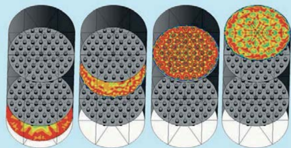
Fig 1: CFD of urea reactor with SuperCups
