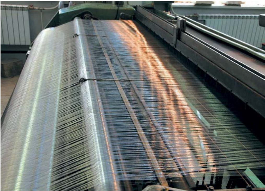
SAFINA catalyst gauze knitting process.
