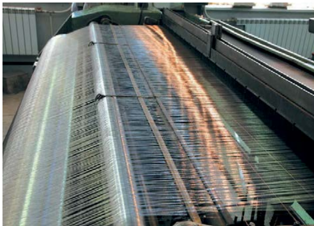
SAFINA catalyst gauze knitting process.
