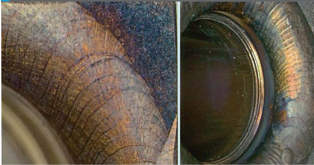
Fig 6: Tube sheet after corrosion: a) weld and HAZ; b) inner surface and zr interface
