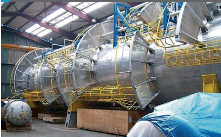
Fig 10: Hydrorested absorption tower dressed in one piece
