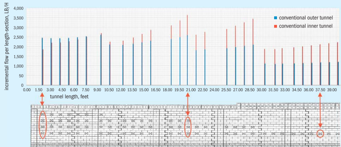
Fig 9: Incremental flow per open-area column for conventional inner and outer tunnels
