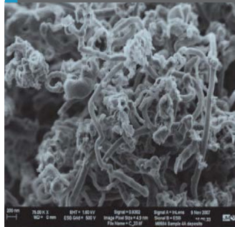
Fig 17: SEM image showing whisker carbon
