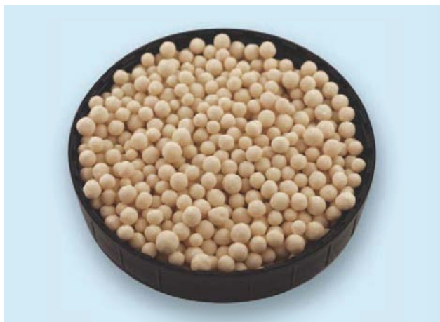
Urea-ES sulphur-enhanced urea (43-0-0 7S), granulated with UFT's fluid bed granulation technology.
