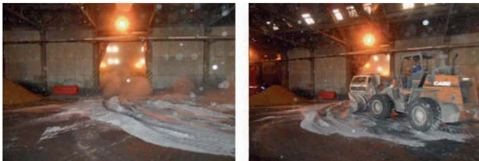
Fig. 4: Near miss of a truck coming out of dusty cloud with an approaching pay loader at NPK plant in Brazil, South America.
