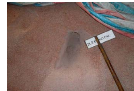
Fig. 10: 21-7-18 NPK with surface crust.
