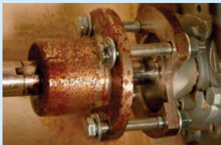
Above left: Failure due to carbon build up.
