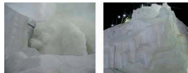
Fig. 3: Urea lumps (left) and severely caked storage pile (right).
