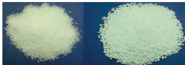
Fig. 1: Typical prill (left) and typical urea granule size (right).
