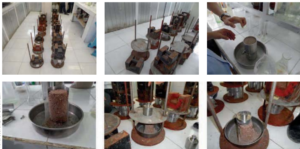
Fig. 7: Company internal caking tendency method at an Asian NPK facility.
