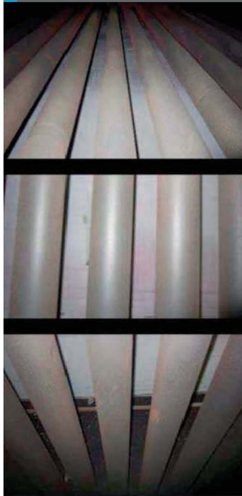
Fig 16: Outer surface condition along the tube length for HP-microalloy catalyst tubes
