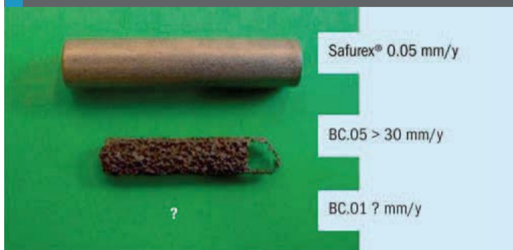
Fig 2: Zero oxygen corrosion test in autoclave 4
