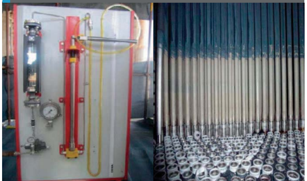
Fig 8: Air test device (left) and leak test of tubes by water level (right)
