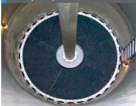
Fig 2: Showerhead™ loading gives higher ammonia catalyst density
