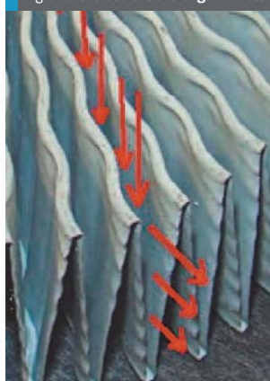
Fig 3: Gas forced out of triangular ducts
