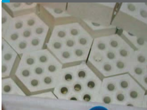
Fig 3: KATALCO JM 94-1 target tiles exposed to high temperature
