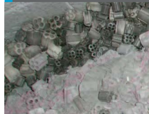
Fig 5: KATALCO JM 89-6 in clean condition alongside alumina catalyst after fouling incident
