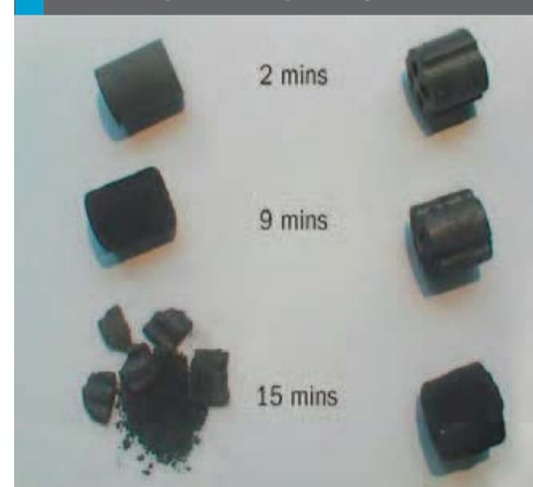
Fig 1: KATALCO JM 46-3 and 46-3Q exposed to pure cyclohexane
