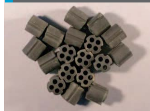
Fig 4: KATALCO JM 89-6 catalyst exposed to high temperature
