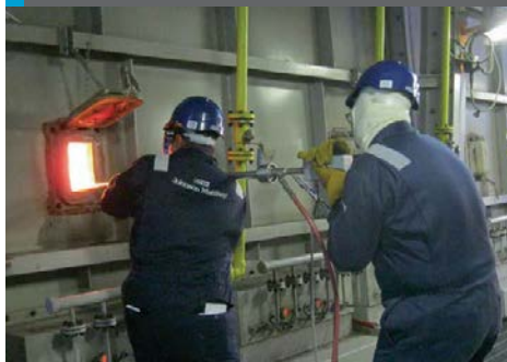
Fig 5: Measuring TWTs with a gold cup
