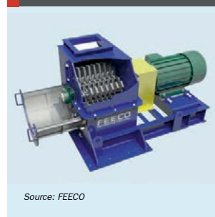
Fig. 5: 3D model of a FEECO hammer mill
