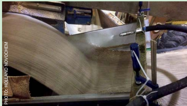
Spray coating fertilizer on a conveyor belt.
