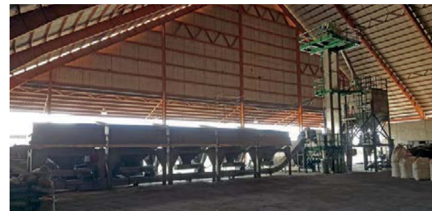
Sackett-Waconia Precision Horizontal Blending system for Mayafert, Guatemala.
