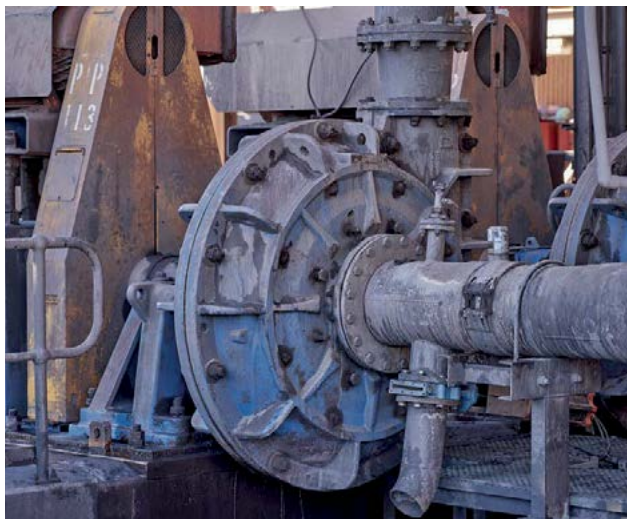
An operational Warman® centrifugal pump.
