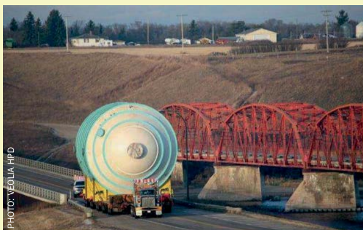
Veolia's KCl crystalliser being transported to the project site.
