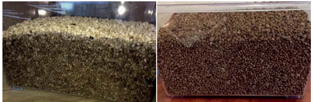
DAP fertilizer made in the same plant, at the same time, under the same conditions. Whitened sample (left): kept under roof but exposed to humidity. Non-whitened sample (right): kept in a climate-controlled office and not exposed to humidity.
