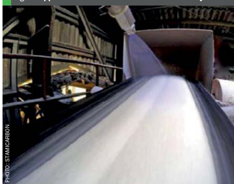
Fig. 4: Application of ADVANCE COAT™ on a conveyor
