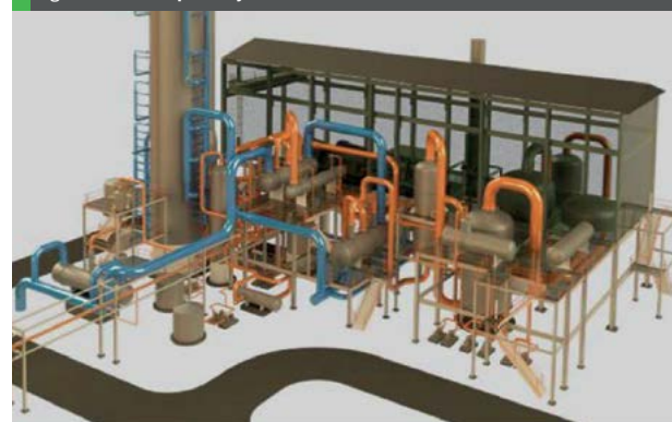
Fig. 7: Nitric acid plant layout
