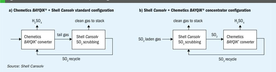
The Shell Cansolv unit can be positioned downstream of the Chemetics BAYQIK® unit in traditional tail gas treatment (standard configuration, Figure 6a). In other applications, the value of combining the two technologies requires placing the Shell Cansolv unit upstream of the Chemetics BAYQIK® unit, where it serves as an SO<sub>2</sub> concentrator while still treating the tail gas (concentrator configuration, Figure 6b).
