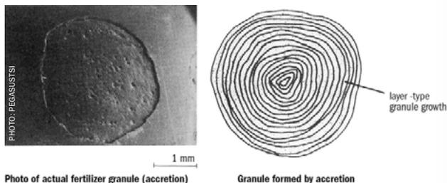
Fig. 3: Granulation by accretion/layering.
